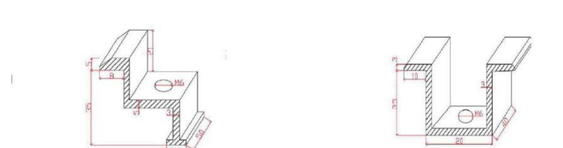
Clamp A for tail end module edge Clamp B for middle modules
