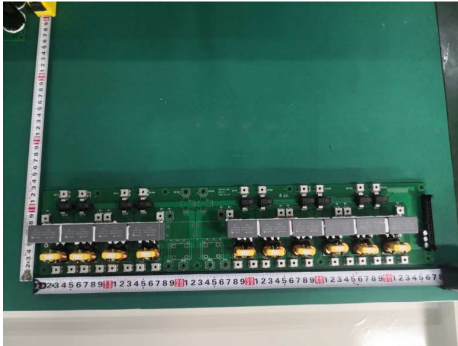
DC EMI board view(Components side)
